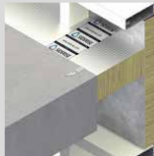
Siderise vertical and horizontal barriers for curtain walling.
